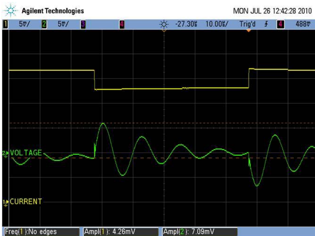
Figure 3. Measured small-signal step-load response (4 mA step) of an LM317T-based regulator circuit with 3.3-V output, 6.3-V input, and a 1-µF capacitor.
