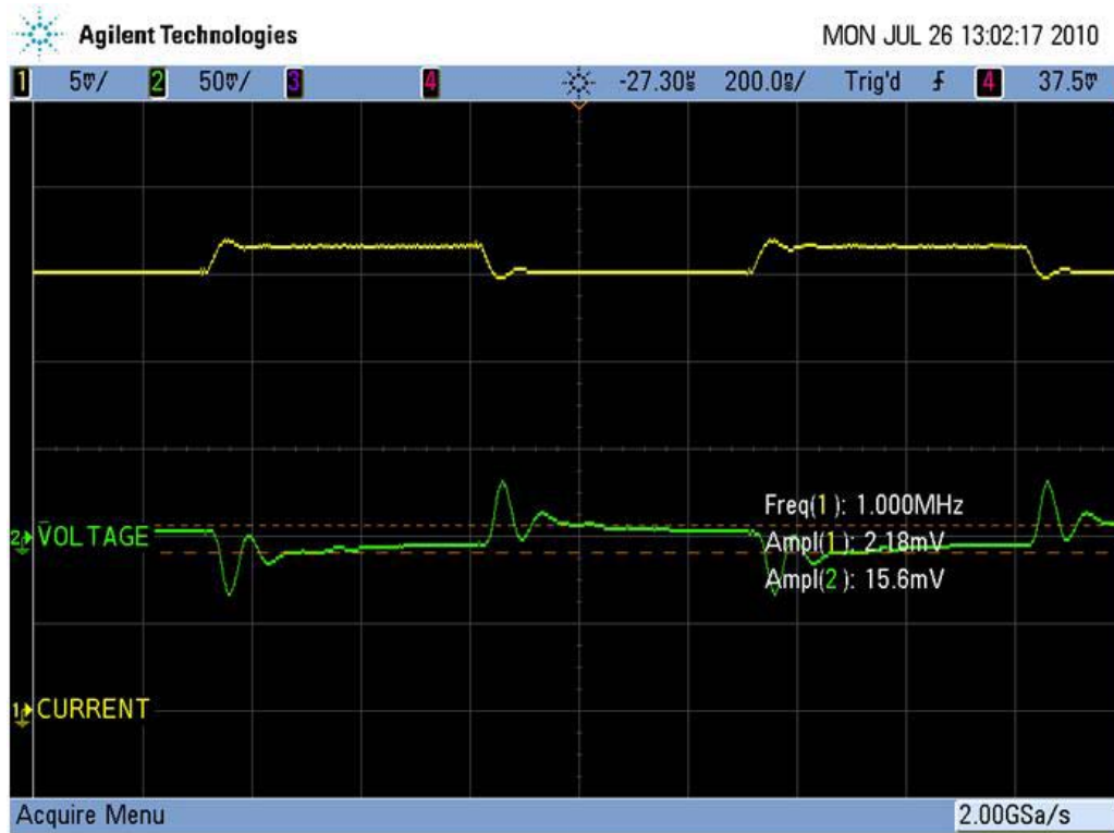
Figure 2. Measured small-signal step-load response (2 mA step) of an LM317T-based regulator with 3.3-V output, 6.3-V input, and no capacitors.
