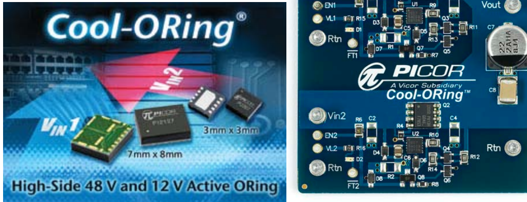
Fig 1. The PI2007 and PI2127 are high-side active ORing devices aimed at 12-V and 48-V high-side intermediate bus applications. The PI2007 is a universal high-speed active ORing controller designed for use with n-channel MOSFETs. The PI2127 co-packages the '2007 controller with a 60-V MOSFET to provide a highly compact active ORing solution. (Devices are shown on left, evaluation board on right.)
