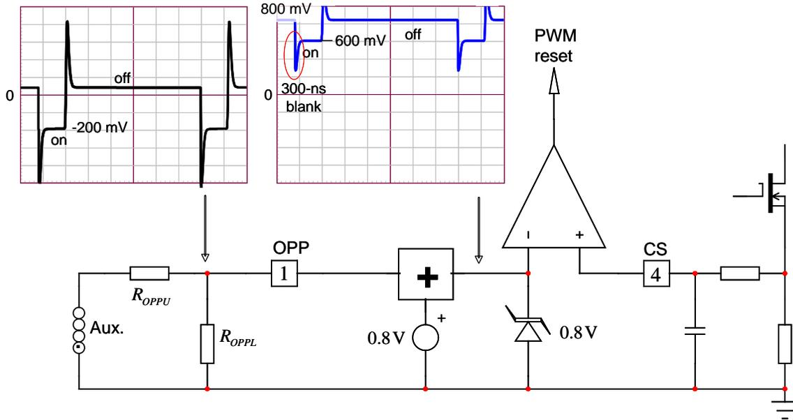
Fig. 9. Sensing the auxiliary winding of the flyback converter during the on time is an excellent way to obtain an image of the input voltage without incurring additional power dissipation.
