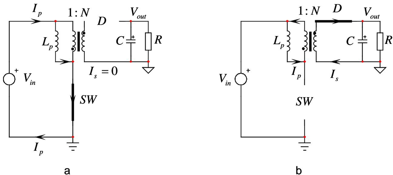
Fig.1. The two operating states of a flyback converter show energy storage in the primary side (a) followed by energy circulation in the secondary side (b).
