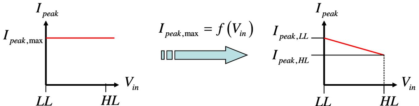
Fig. 6. One approach to implementing over-power protection is to limit the peak current as a function of input voltage.
