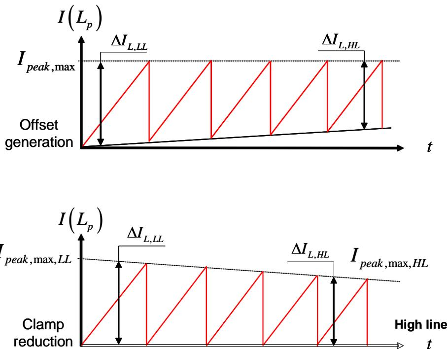
Fig. 7. The reduction in the peak-current limit at high line can be obtained by either offsetting the current-sense signal (top graph) or by reducing the internal clamping value (bottom graph).
