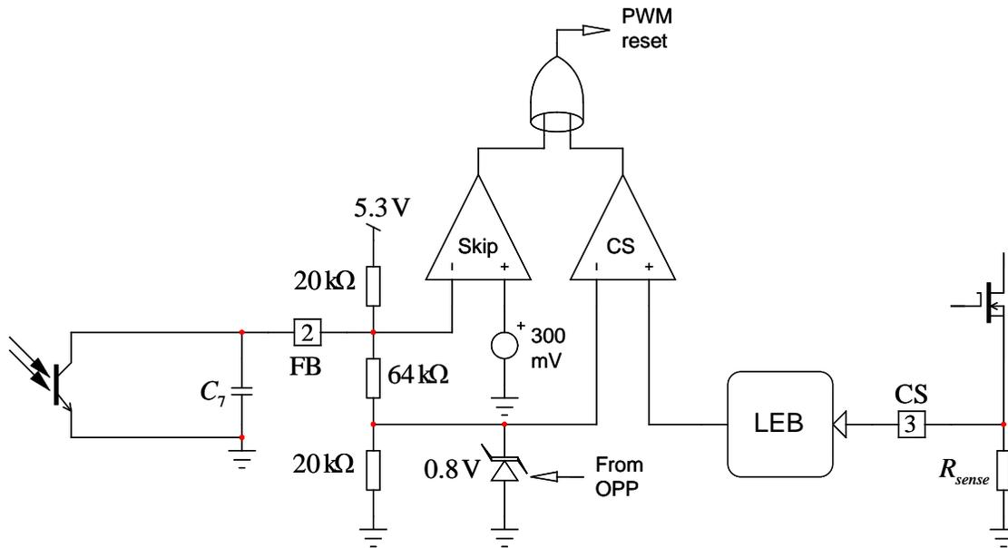
Fig. 4. The maximum peak current is set by the 0.8-V reference voltage.
