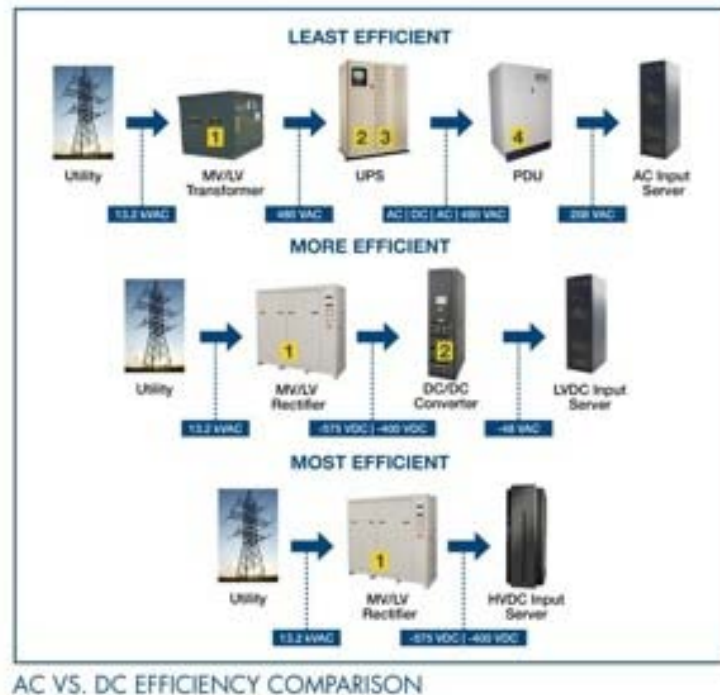
Fig. The energy losses associated with today's ac power systems come from the rectifications and inversions that are required to reliably deliver ac power to dc equipment in data centers. Validus's dc system provides an energy efficient power path that eliminates losses associated with traditional ac systems.
