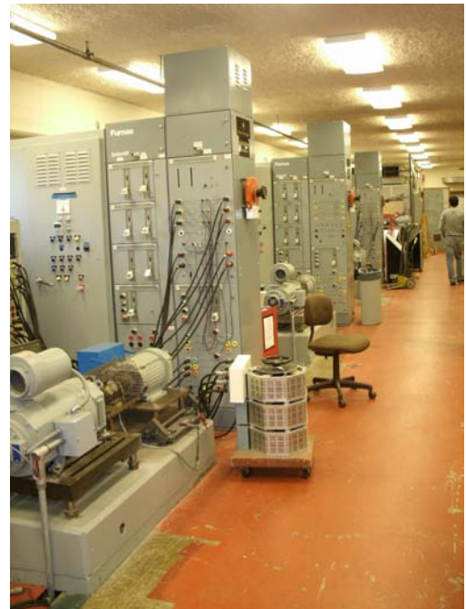
The Emerson Electric Company's Drives Laboratory offers access to general-purpose dynamometers and a two-dynamometer system for emulating electric vehicles.
