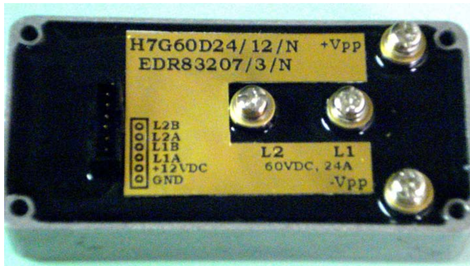
Fig. 1. Assembled in a 1.95-in. (W) x 3.95-in. (L) x 1.2-in.(H) panel mounting enclosure, the H7GvvDcc/v/T high-power full bridge drivers are guaranteed to deliver 4.5 kW continually (30 kW pulse).
