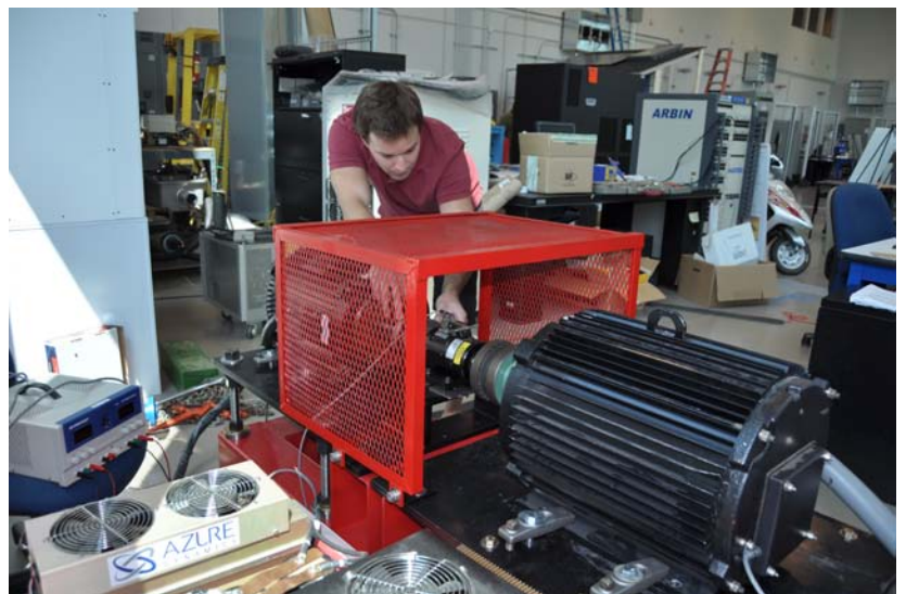
Josh Lawrence, a mechanical engineering graduate student at the FREEDM Systems Center, makes adjustments to the electric dynamometer—a key piece of equipment in his research.
