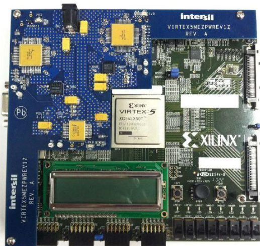
Fig. 4. Intersil's rad hard FPGA power solutions reference design board, the VIRTEX5MEZPWREV1Z board, is optimized to power a Xilinx's Virtex-5 FPGA using rad hard components such as the ISL70001SRH and ISL70002SRH POLs and the ISL75051RH LDO.
