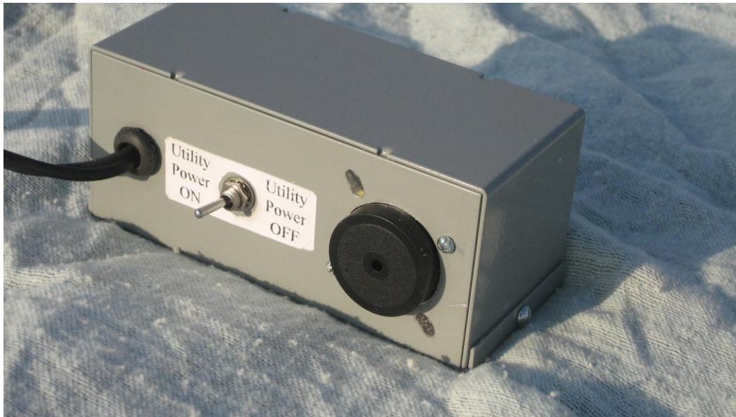
Fig. 1. Throwing a switch on the front panel activates the monitor so that it will generate a sound when utility power fails and also when the power returns.
