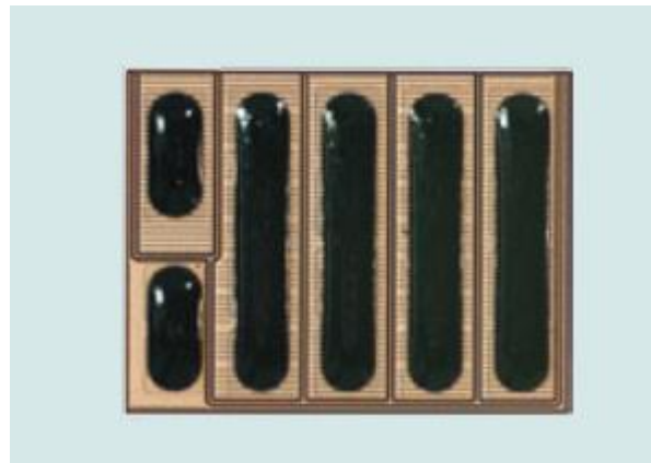
Fig.1. EPC's eGaN FETs are offered in die form to cut package cost and parasitics.
