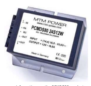
The converters are available with three wide input ranges thus covering the battery voltages of 24 V, 36 V, 48 V, 60 V, 72 V, 80 V, 96 V and 110 V in accordance with EN 50 155. The dimensions of the base plate version are 119 x 100 x 40 mm and of the heatsink version are 119 x 115 x 65 mm. The thermoselective vacuum encapsulation guarantees homogeneous heat dissipation within the modules as well as an excellent resistance against environmental influences such as shock, vibration and humidity.
