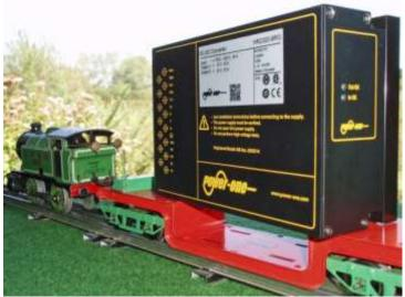
The converters are particularly suitable for railway applications and can be operated from all common dc traction supplies of 24 V, 36 V, 48 V, 72 V, 96 V, 110 V and 120 V nominal. The output is configurable as 12 V,  $\pm 12$  V or 24 V. The converters comply with EN51055 and EN50121-3-2, IEC/EN 60950-1, IEC61000-4-2, -3, -4, -5, -6. The HR2320-9RG is Network Rail approved, certificate number PA05/05958 catalogue number 086/034203.
