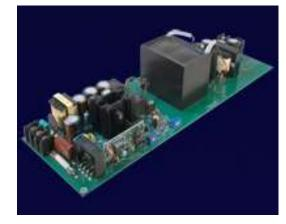
between primary and secondary is 2 to 5 kV rms. This value depends on the specific application and contamination class, and is limited by the creepage distance of 76 mm (3.0 in.) on the PCB.
