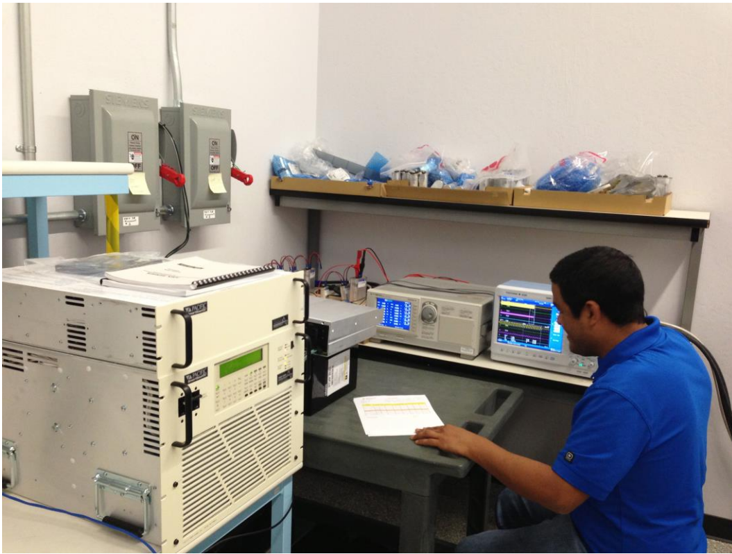
Figure. An inverter undergoing anti-islanding testing in TÜV Rheinland's inverter testing lab in Pleasanton, Calif.
