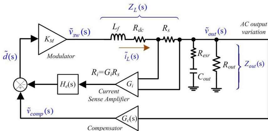
Fig. 3. Simplified small-signal control loop block diagram of a buck converter with peak current-mode control.  $H_e(s)$  is the sampling gain block in the current loop.
