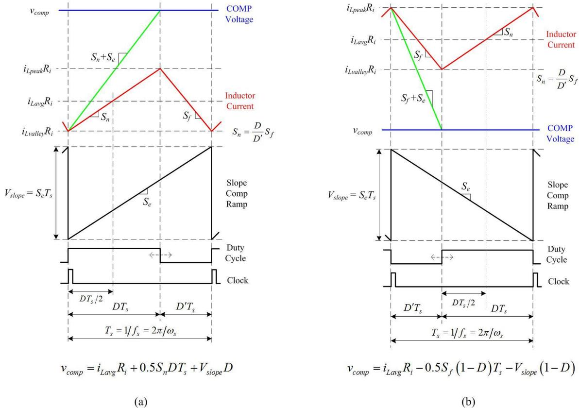
Fig. 2. Modulator waveforms and timing for peak (a) and valley current-mode control (b).
