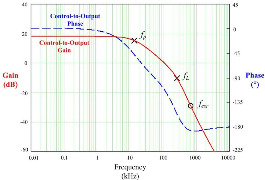
Fig. 4. Typical buck converter control-to-output small-signal frequency response.
