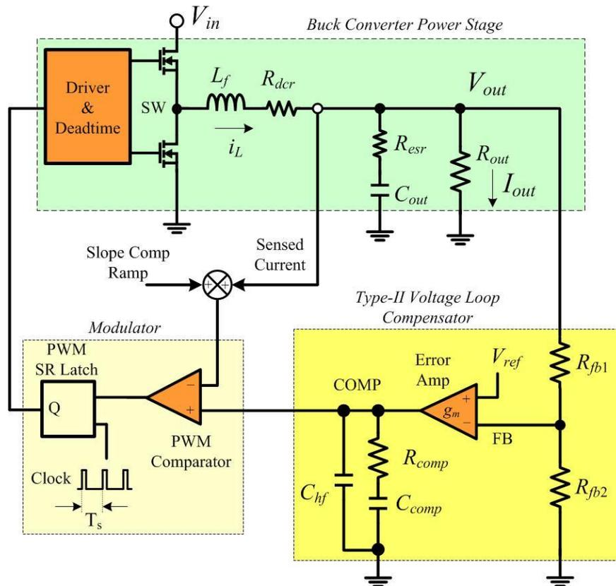
Fig. 1. Dc-dc synchronous buck converter schematic of power train, driver stage and peak/valley current-mode PWM control loop structure with transconductance error amplifier.
