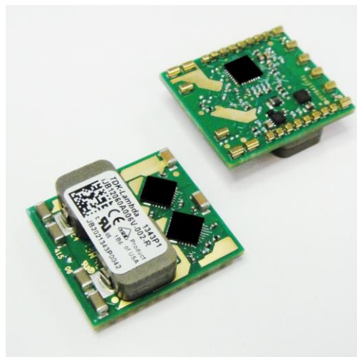
Fig. 1. The 60-A iJB series point-of-load converters (POLs) feature intelligent auto-tuning technology that enables better dynamic performance and improved system stability. These PMBus-enabled units, which measure just 1.05 in. x 0.95 in. x 0.381 in., also provide real-time monitoring of voltage, current and temperature.
