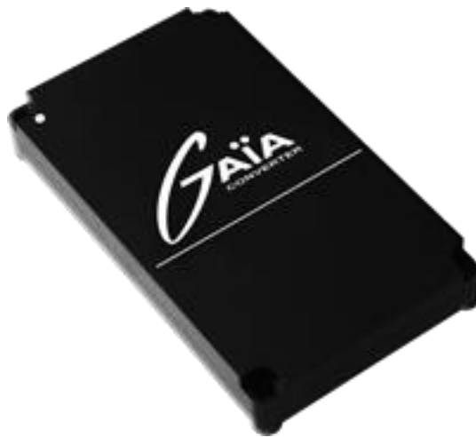
Figure. Targeting military and airborne applications, the MGDD-60W series 60-W dc-dc converters feature a 12-V to 160-V input range that enables compliance with Mil-Std-1275 (even the strict Mil-Std-1275E version), 704 or DO-160 standards without requiring an additional front end protection device.
