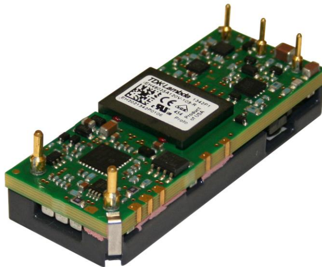
Fig. 2 These eighth-brick converters, which include a baseplate with mounting holes for an external heatsink, deliver up to 192 W of output power with only 200 LFM of airflow in an 85°C ambient.
