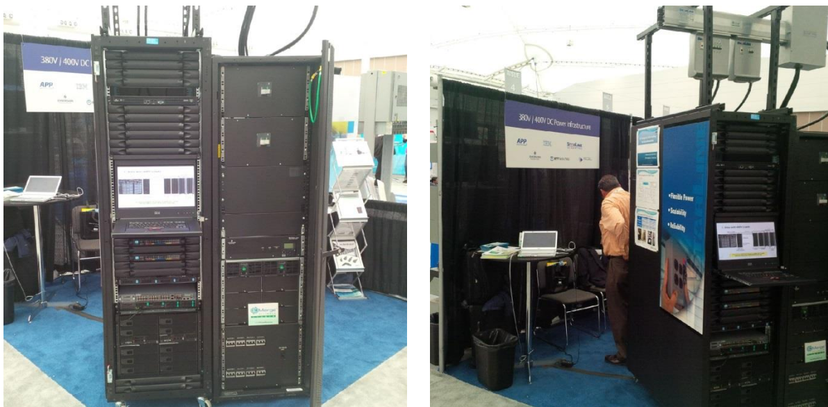
Fig. 2. Front and side views of the two equipment racks in the HVDC power system demo at INTELEC 2014.
