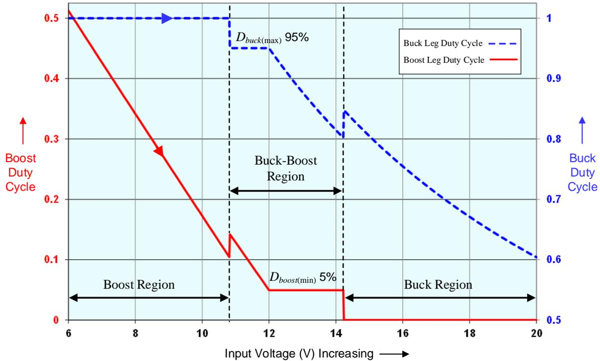
Fig. 4. Buck and boost leg duty cycle variations over the input voltage range. Output voltage is 12 V.
