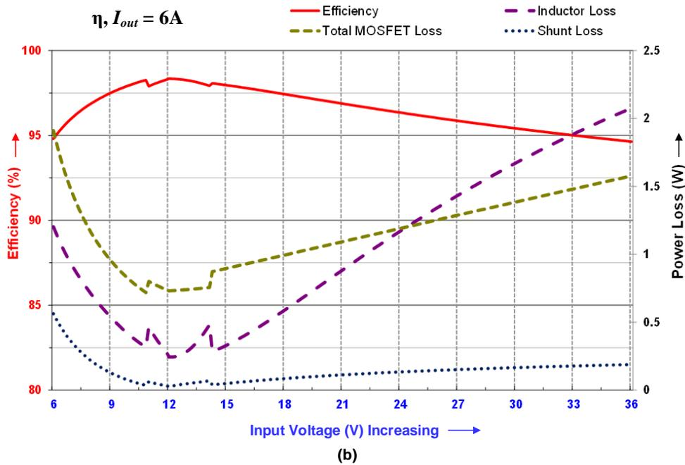
Fig. 6. Efficiency plots and component power loss breakdown versus load current (a) and input voltage (b). The buck-boost window is evident in the efficiency vs. line plot.
