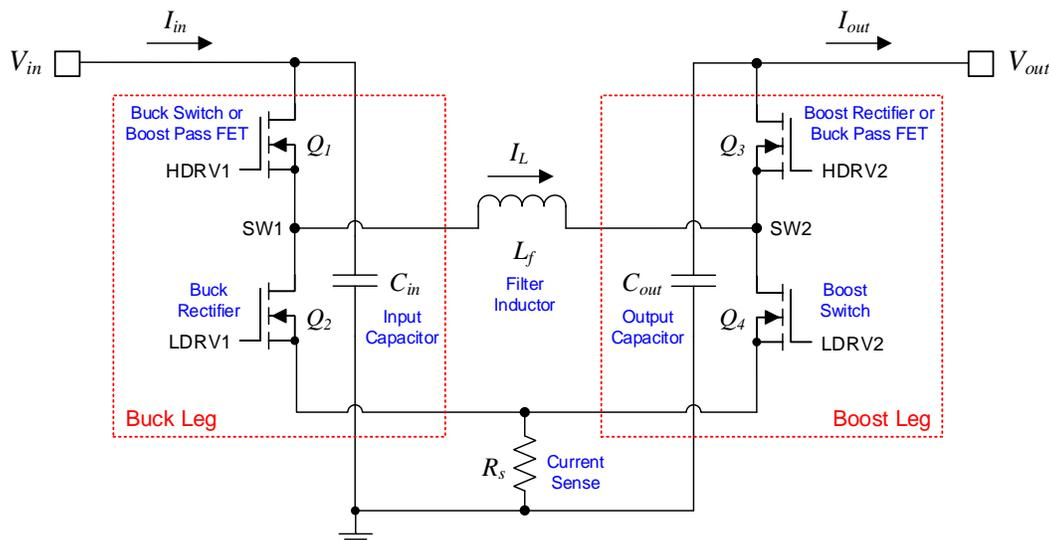
Fig. 1. Four-switch synchronous buck-boost converter power stage. Three operating modes are possible depending on the input voltage relative to the output voltage: buck ( $V_{IN} > V_{OUT}$ ), boost ( $V_{IN} < V_{OUT}$ ) and buck-boost transition ( $V_{IN} \approx V_{OUT}$ ) mode.
