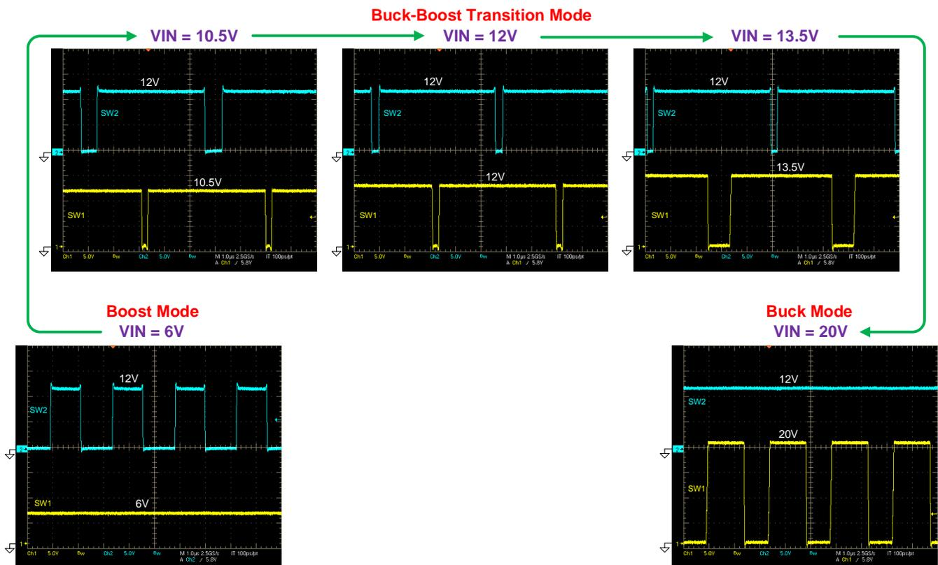
Fig. 2. SW-node voltages for buck (SW1) and boost (SW2) legs during buck, boost, and buck-boost operating regions.  $V_{out} = 12\text{ V}$ .
