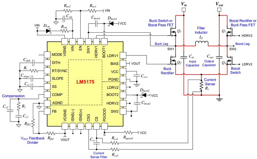
Fig. 5. Practical four-switch buck-boost converter schematic with peak/valley current-mode controller.
