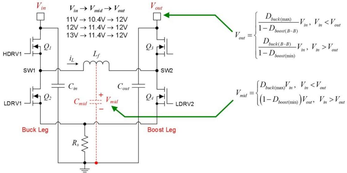
Fig. 3. This equivalent circuit model for power stage operation in the buck-boost region is used to derive duty cycle equations.
