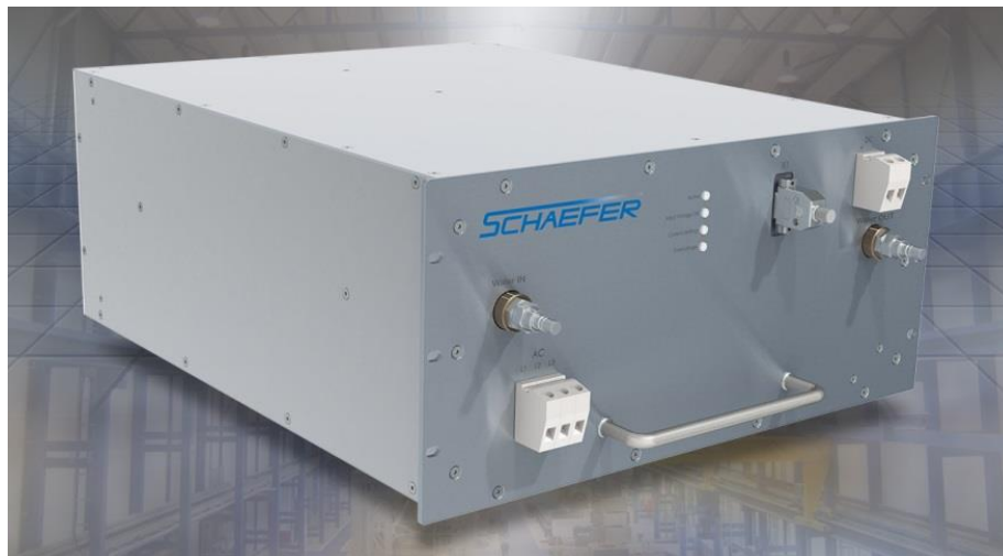
Figure. The CPW-5700 series of ac-dc supplies and the BPW-5700 series of battery chargers are robust, shock resistant liquid-cooled power supplies designed for the harshest operating conditions in industrial and military applications. They feature three-phase, wide-input ranges for 200/400/440 V ac and 480 V ac and selectable output voltages and currents.
