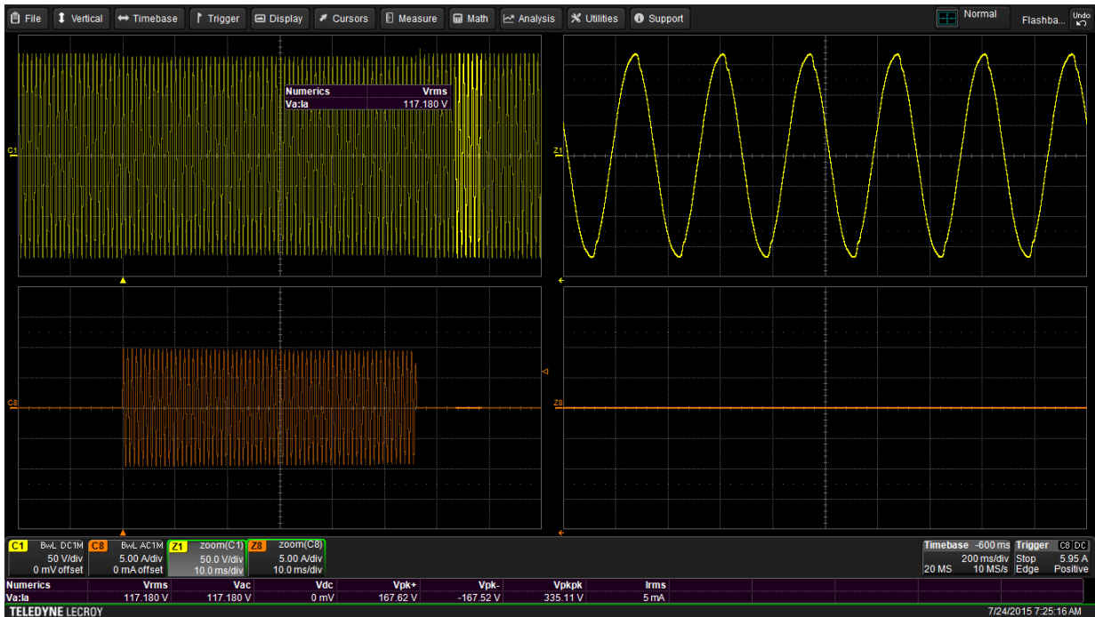
Fig. 9. AC line measurements with toaster load off.
