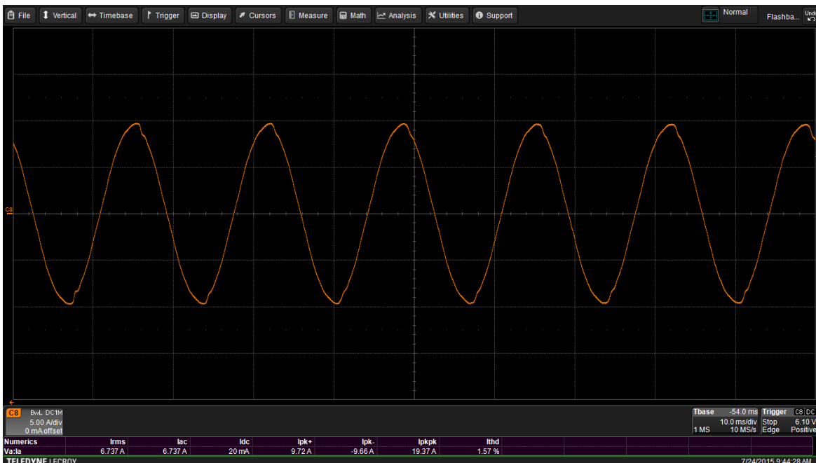
Fig. 3. 120-Vac current signal captured with a Teledyne LeCroy 8-channel, 12-bit Motor Drive Analyzer. This measurement is identical to the voltage measurement of the 120-Vac signal in part 2, except for the use of a current probe in place of a high-voltage probe.
