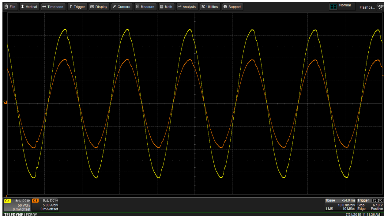
Fig. 5. 120-Vac current (orange trace) and voltage (yellow trace) waveforms captured with a Teledyne LeCroy 8-channel, 12-bit Motor Drive Analyzer. The two signals are in phase as expected with a resistive load.
