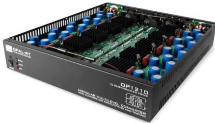
OPAL-RT's Lab-Scale Multilevel Modular Converter test bench.
