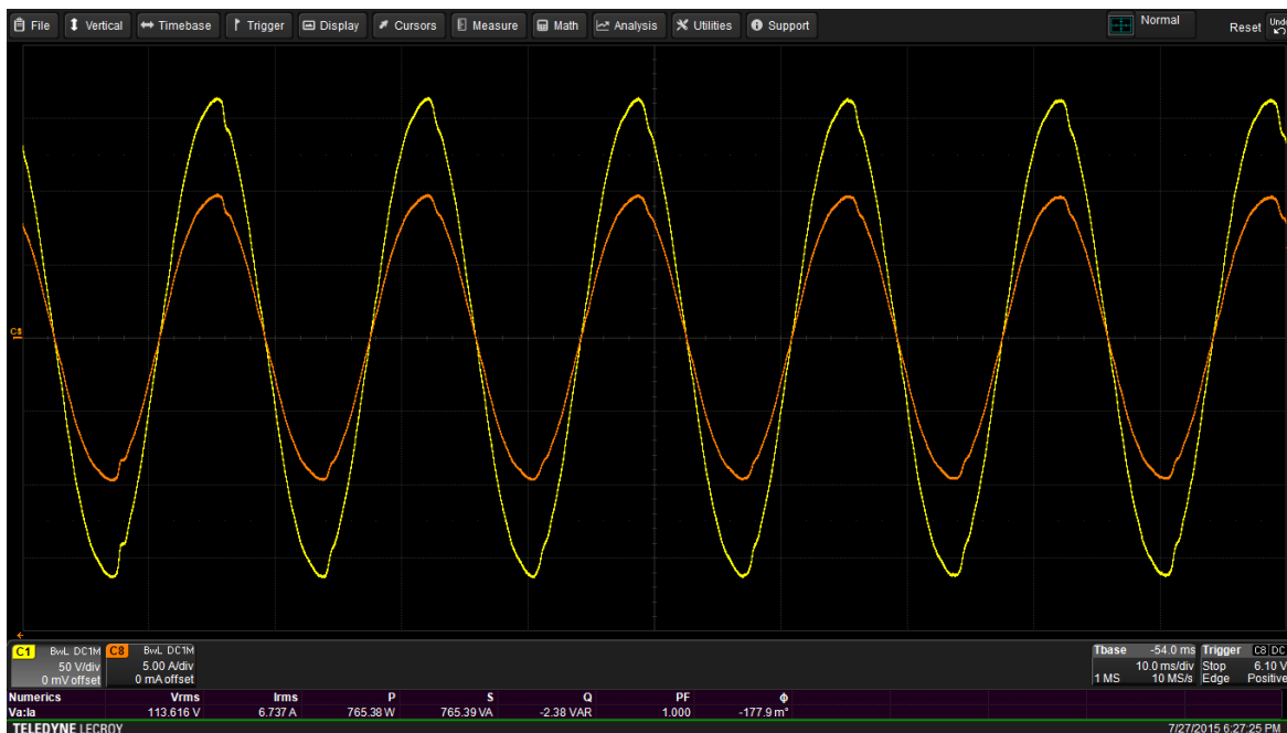
Fig 12. Line-to-neutral voltage waveform and the associated current waveform for a linear load are shown with the Numerics calculation table, which displays various power-related parameters for these waveforms.
