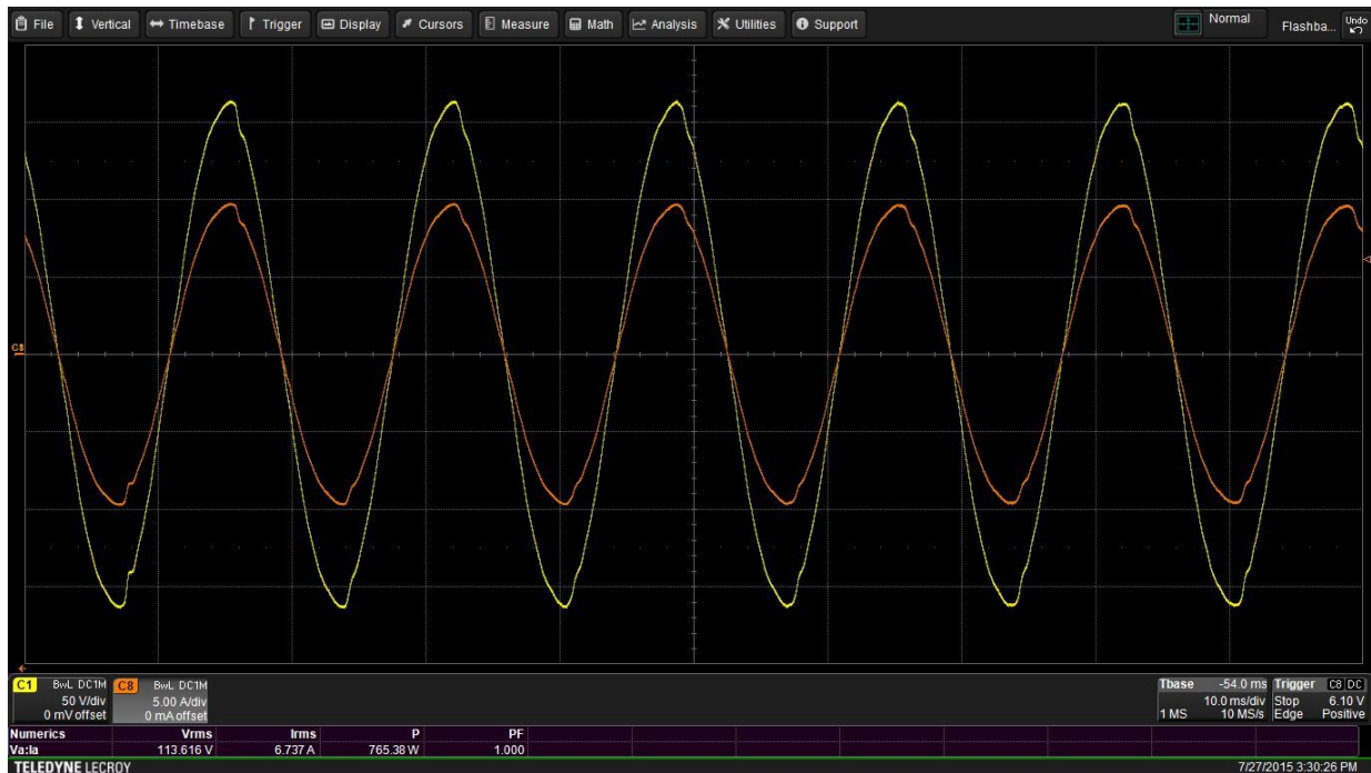
Fig. 2. Line-to-neutral voltage waveform and the associated current waveform for a linear load captured with a Teledyne LeCroy 8-channel, 12-bit Motor Drive Analyzer.
