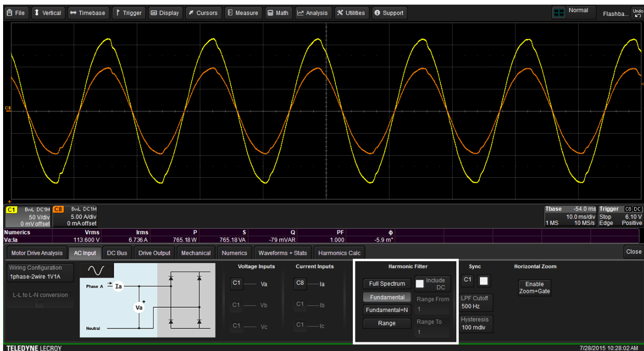
Fig 14. Voltage and current waveforms with power measured for just the 60-Hz fundamental. Apparent and real power are equal and phase angle is zero. This suggests that the visible distortion in the waveforms is due to some complex impedance in the load at higher frequencies.
