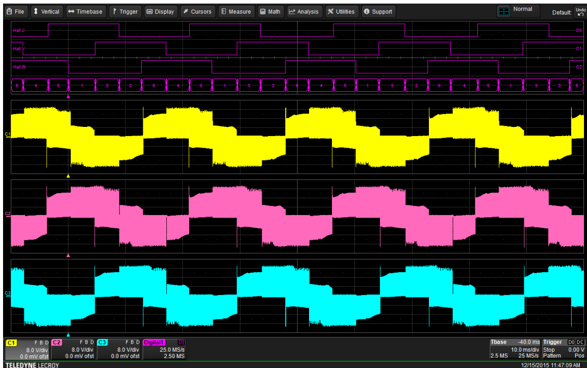
Fig. 9. Line-to-line six-step commutated voltages signals together with their three Hall sensor signals.
