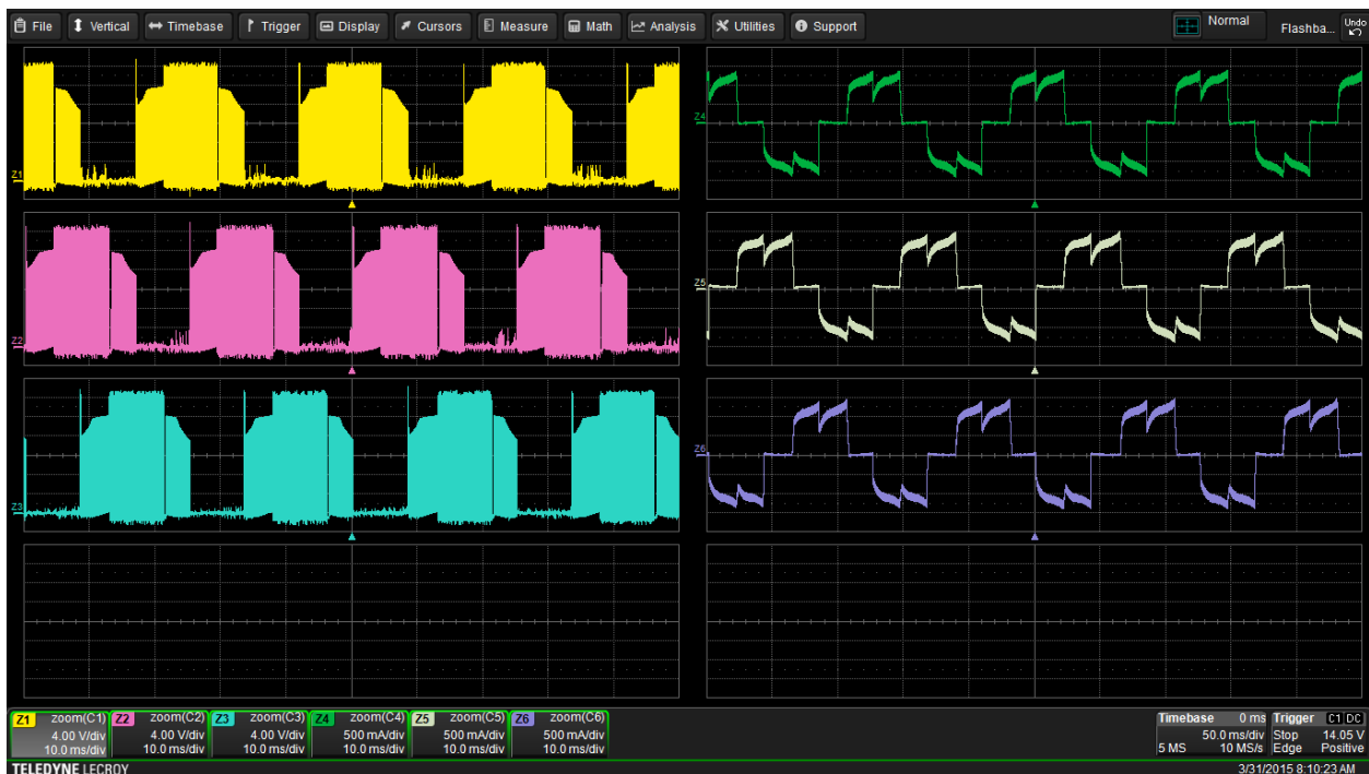
Fig. 6. Six-step commutation control produces the motor drive line-to-reference output voltages (waveforms on left) and currents (waveforms on right) shown here. The back-EMF influence from a nearby (energized) phase on the adjacent (non-energized) phase results in the "ramp up" or "ramp down" of the peak voltage, and thus the trapezoidal shape.
