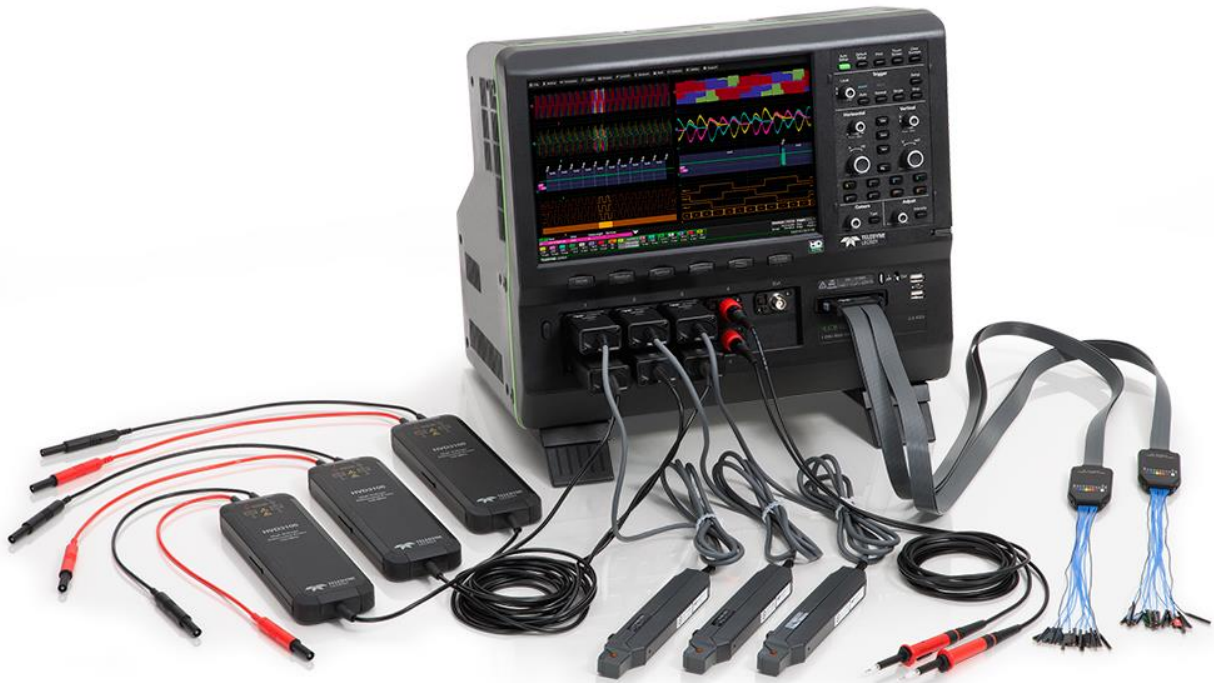
Fig. 3. Featuring eight analog channels and 16 digital inputs, Teledyne LeCroy's MDA800 series oscilloscope can handle the large number of signals that must be monitored at one time for proper debug and characterization of a VFD control system.
