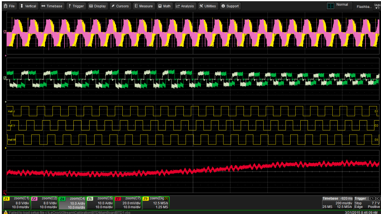
Fig. 10. Two of three line-to-line drive output voltages (Z1, yellow and Z2, magenta) with drive output motor line-currents (Z4, gray and Z5, green); digital Hall-sensor signals (Hall U, V, and W, yellow traces); and torque sensor signals (Z7, red) are shown for a six-step commutated closed-loop (sensored) control system.
