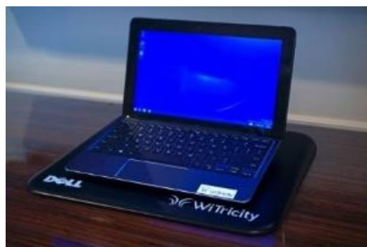
Fig. 1. Dell's 2-in-1 Latitude computer is wirelessly charged using a highly resonant magnetic power-transmitting unit (PTU) based on the AirFuel standard.
