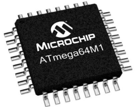
Microchip Technology's ATMega64M1 rad tolerant, general-purpose, 8-bit, 8-MHz, RISC-based microcontroller.
