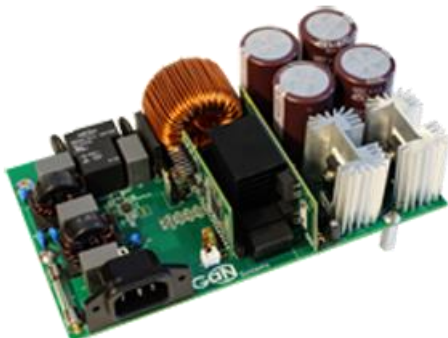
GaN Systems' 3-kW PFC reference design.
