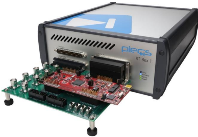
Plexim's RT Box simulator for real-time hardware-in-the-loop testing and rapid control prototyping.
