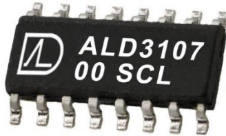
Figure. Intended for low-voltage and low-power small-signal applications, the ALD310700A/ALD310700 features precision 0.00-V zero-threshold voltage, which enables circuit designs with very low operating voltages such as < +0.5-V power supplies where the circuits operate below the threshold voltage of the ALD310700A/ALD310700. A sample device and pinout are shown here.
