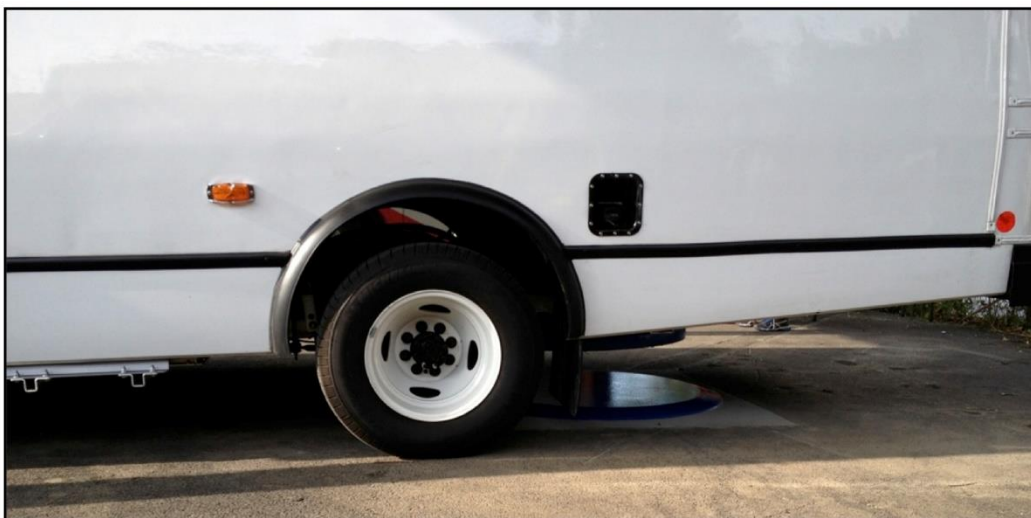
Fig. 14. A high-power WEVSE GA for HD vehicle charging (courtesy of Momentum Dynamics).
