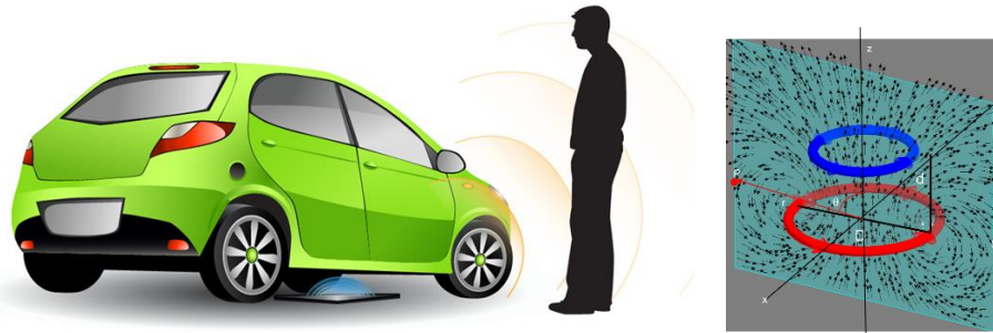
Fig. 13 Illustration of leakage EMF (graphic courtesy Oak Ridge National Laboratory) and coupler field pattern (graphic courtesy of the University of Texas-Dallas (UTD) and [11]).
