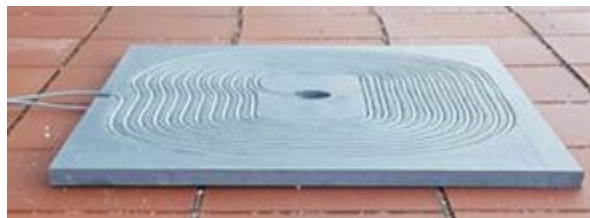
Fig. 2. Charging module for 22-kW wireless charger.
