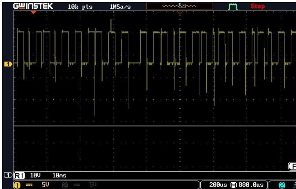
Fig. 9. Magnified phase-phase output voltage waveform.
