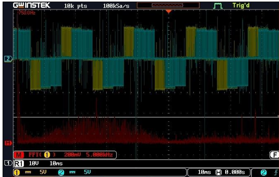
Fig. 11. V_{ab} , V_{ac} and FFT for a reference value of 0.5.
