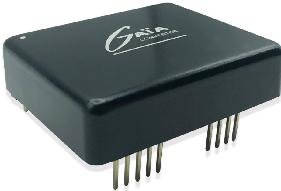
Figure. Featuring an input voltage range of 9 to 60 V, the MGDD-80 series dc-dc power modules are designed for use in distributed power architectures in military and avionics applications where variable input voltage and transients are prevalent and where high power density up to 50 W/in. 3 is required. The MGDD-80 series is compliant with DO-160 and MIL-STD-704 transient voltage without an additional voltage limiter.
