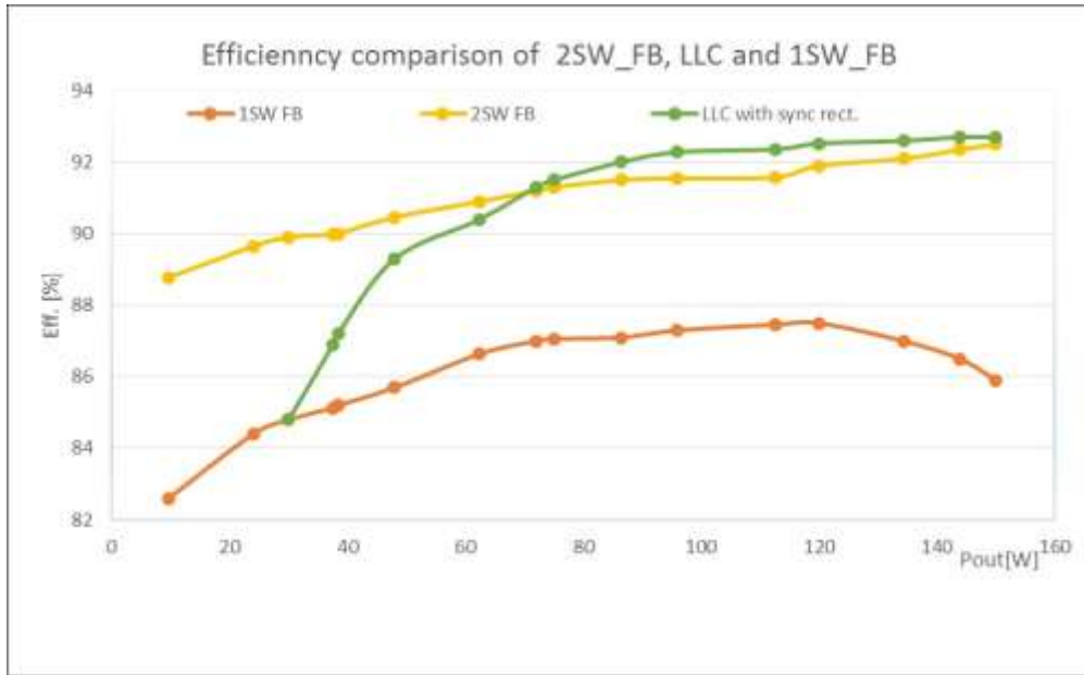
Fig. 3. Efficiency comparison of a two-switch flyback with an LLC resonant and a single-switch flyback.
