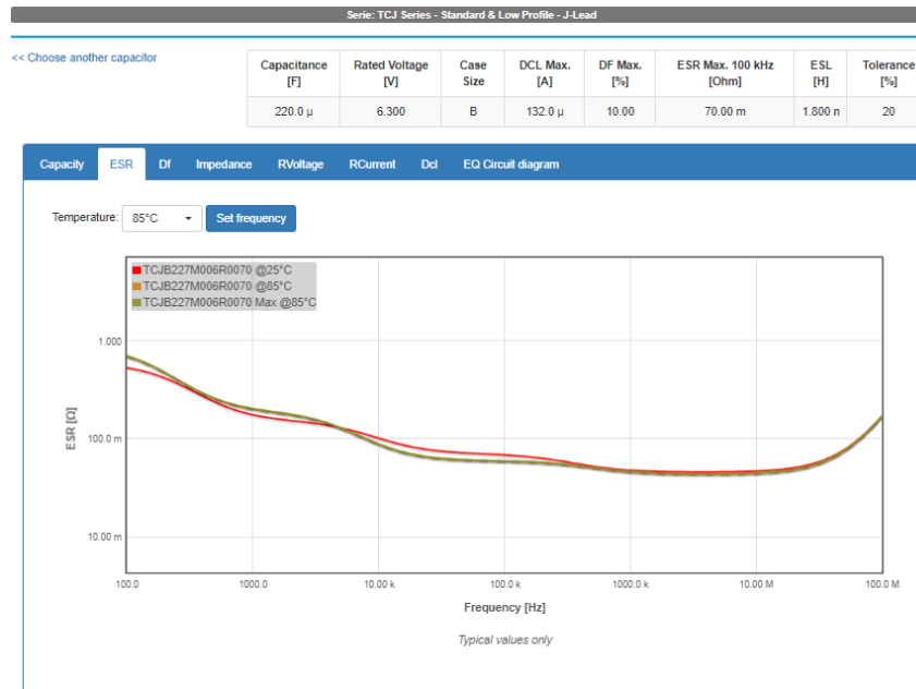
Fig. 9. Example of tantalum polymer ESR simulation.
