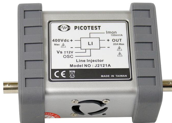
Fig. 1. In combination with a vector network analyzer, the J2121A line injector enables measurement of PSRR, dc biased inductor measurement, dc-dc converter input impedance testing, as well as other EMI tests. The injector is especially suited to high-power applications such as those associated with military and satellite buses. It can be used with input bus voltages up to 400 V and supply up to 20 A at 1 MHz.
