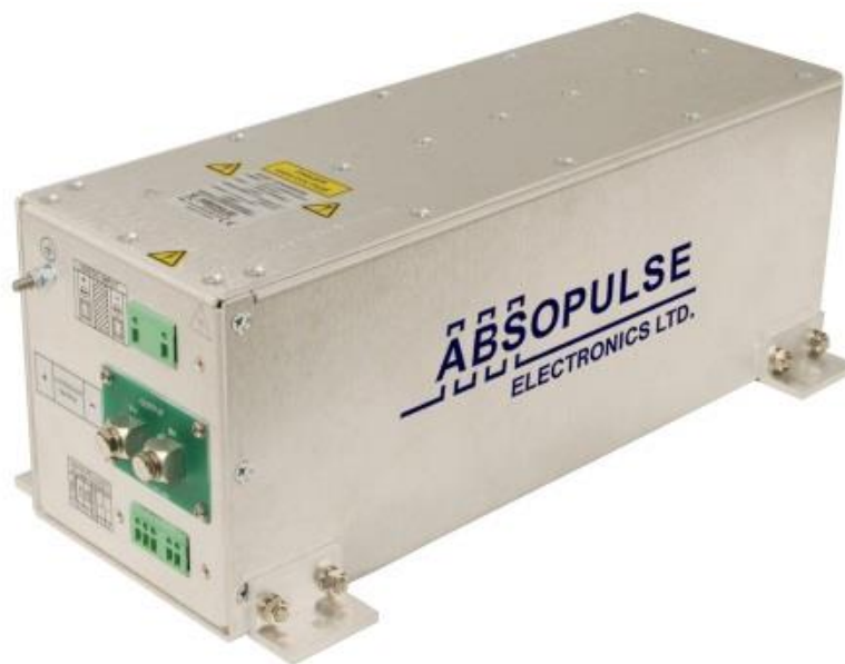
Figure. Measuring 5.2 x 5.8 x 15 in., the LQC 2K-3U2LC liquid-cooled dc-dc converter operates from a wide input voltage range of 400 V to 800 V, while generating a 24-V output at up to 80 A. The output is floating and other output voltages are available on request.
