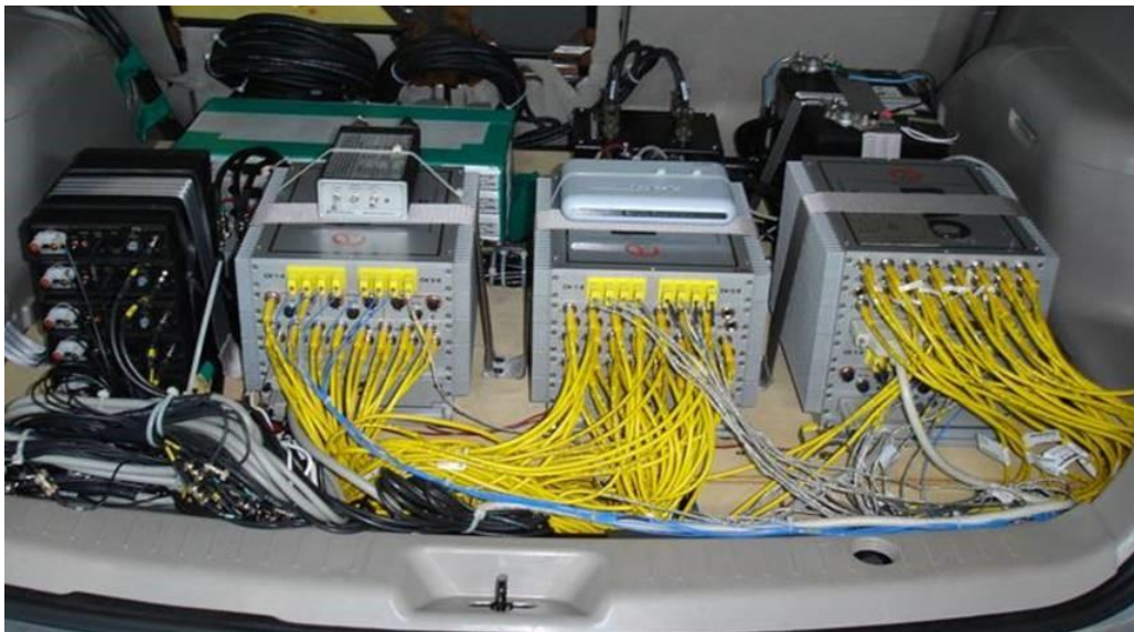
Fig. 1. HBM's eDAQXR data acquisition system is designed for rugged in-vehicle structural measurements.
