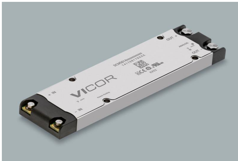
Fig. 1. An isolated, regulated dc-dc converter in Vicor's flat VIA package, the DCM5614 steps down a 270-V input to 28-V output at up to 1300 W with 96% efficiency. Available in chassis- or PCB-mount form-factors, the 5.6- x 1.4- x 0.3-in. module incorporates a dc-dc converter, inrush protection and optional analog or digital communication.
