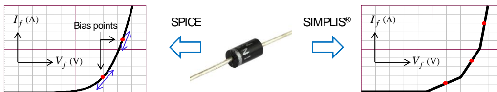
Fig. 12. SIMPLIS uses perfect elements described by linear segments.
