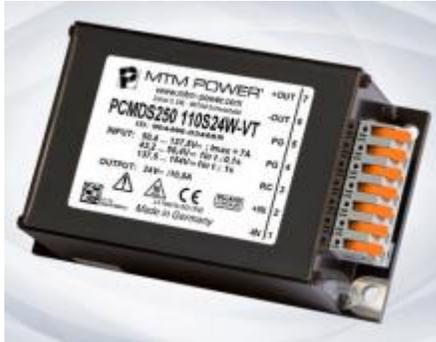
The dc-dc converters are now connected via push-in cage-clamp connectors with lever, which are designed for wire cross sections up to 4 mm<sup>2</sup>. Designed for an operating temperature range of -40°C to + 70°C (class TX according to EN 50155) the cooling is guaranteed either by the integrated heatsink (option WK) or by mounting the baseplate on a heat dissipating surface.
