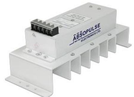
The converters are fully encapsulated with a thermally conductive MIL-grade silicon rubber compound with a UL94V-0 flammability rating. Encapsulation ensures protection from high levels of shock and vibration, moisture, dust, salt, fog and other contaminants. Encapsulation also provides heat dissipation throughout the module.
