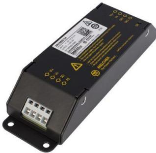
Nominal on-board battery voltages from 24 V to 110 V are covered by one universal ultra-wide input range and converted into a fully regulated and isolated single output voltage of 12 V, 15 V or 24 V. The converters can operate fully loaded in a convection-cooled environment at temperatures from -40°C up to 70°C. All PCBs are conformal coated and protected against humidity and pollution which occurs during typical lifecycles of +20 years of rolling stock equipment.
