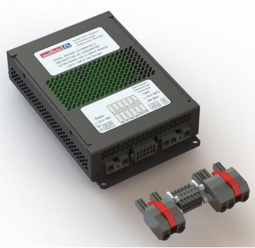
[Murata Power Solutions'](#) IRV300 is a 300-W chassis-mount dc-dc converter with an ultra-wide 10:1 input range, a patented inrush current control topology and a high efficiency of >92%. The IRV300 is a fit-and-forget module designed for harsh operating environments in railway and industrial applications. It conforms to EN50155, EN50121 and EN45545, and has an operating ambient temperature range of -40°C to +85°C.
