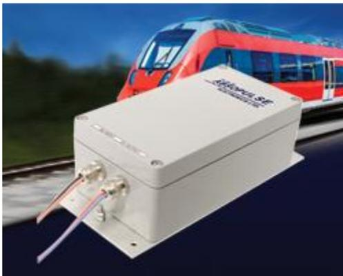
The RSI 100-D1 series uses microprocessor-controlled high-frequency PWM technology to deliver 100-VA pure sine wave output voltage. The inverters convert dc inputs of 24 V, 48 V, 72 V, 96 V or 110 V with wide EN50155 input ranges, to 115 Vac at 60 Hz or 400 Hz, 230 Vac at 50 Hz or a custom output. Regulation is  $\pm 3\%$  from no load to full load.
