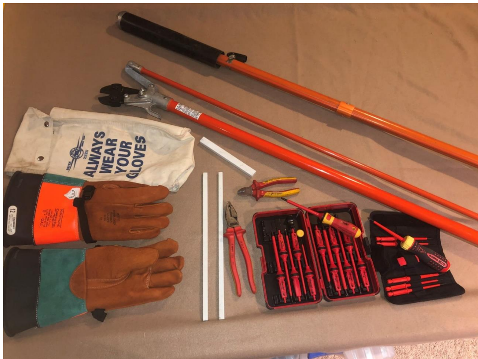
Fig. 2. Tools and insulation for lab tests ranging from 1 kV to 30 kV.
