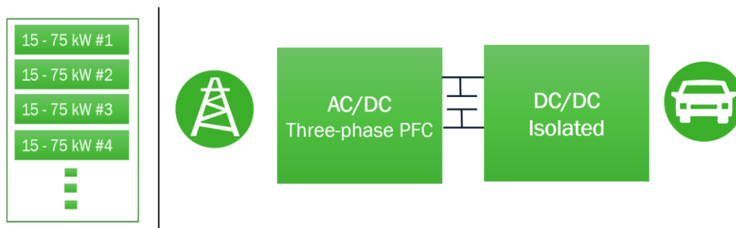
Fig. 1. A high-power fast dc charger with several power stages (left). A high-level architecture of fast EV dc charging systems (right).
