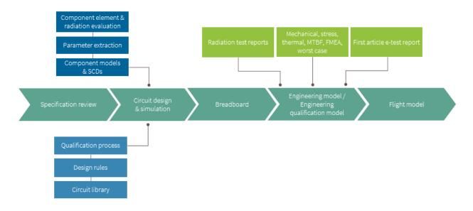
Fig. 1. Design flow to production for IR HiRel's Class K hybrid dc-dc converters.
