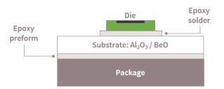
*Fig. 3. A thermal spreading model is used to predict the junction-to-case temperature rise for each of the semiconductor devices in the hybrid assembly.*
