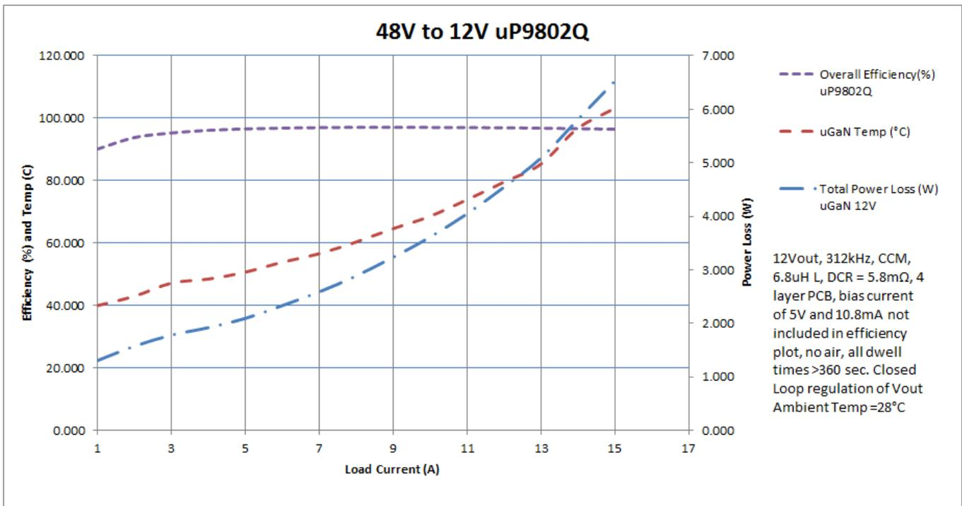
Fig. 7. Overall electrical and thermal performance for the example converter based on the uP9802Q.
