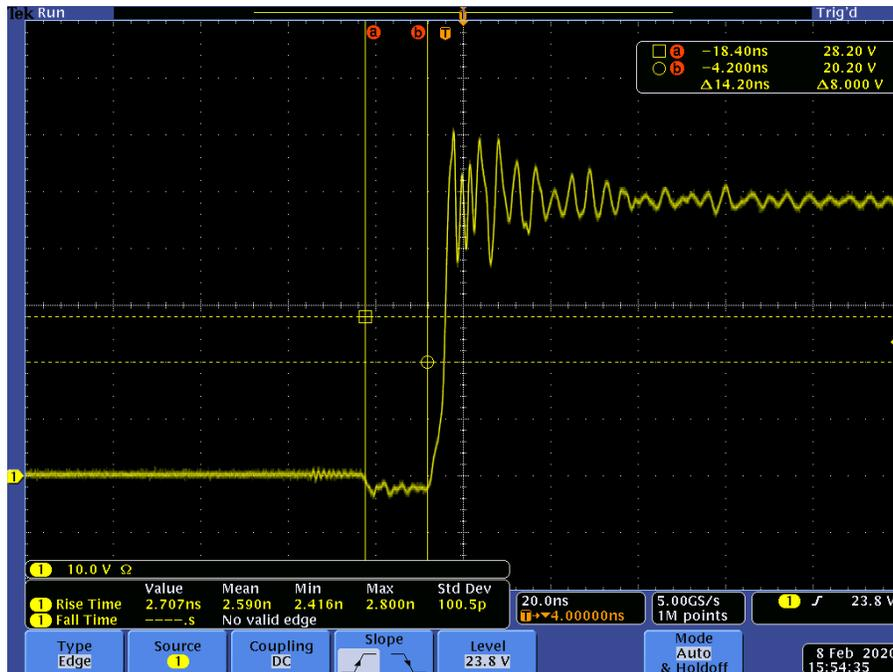
Fig. 12. Rise time and dead time measured for the uP9802Q on the test board.
