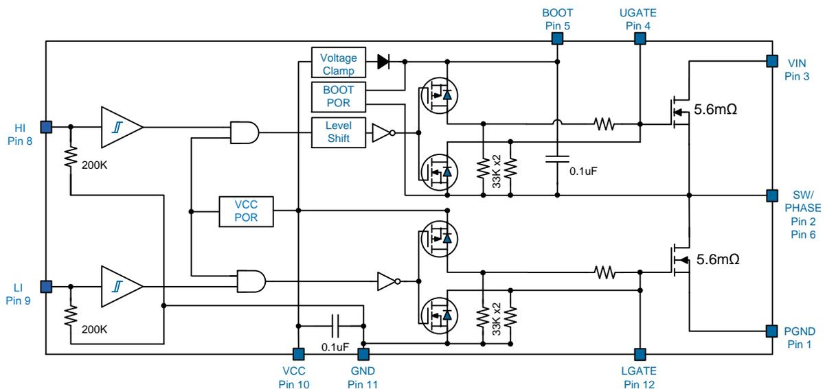
Fig. 1. uP9801Q block diagram.
