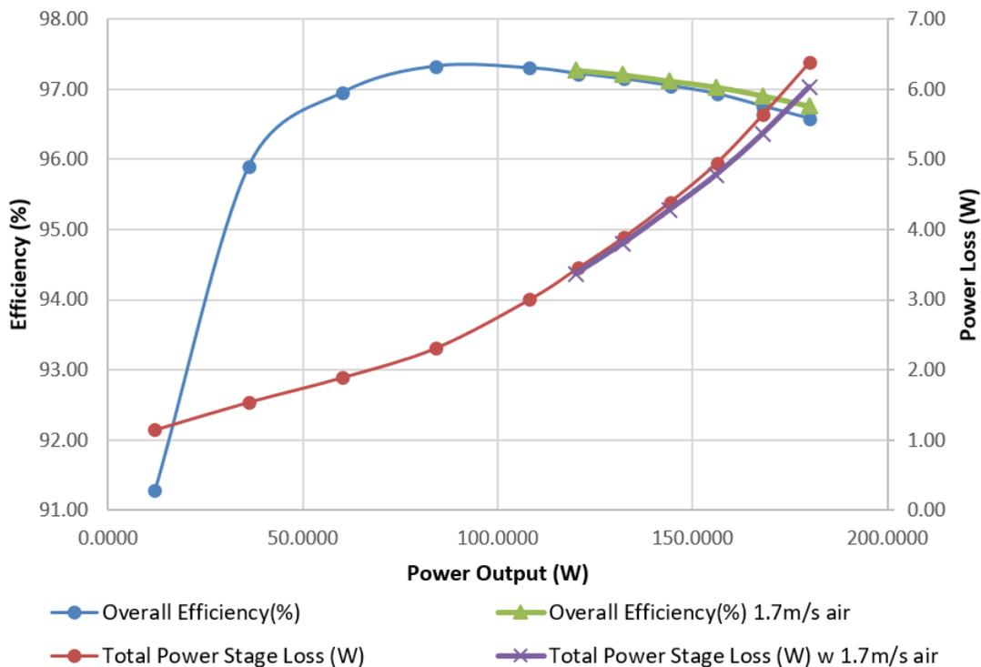
Fig 10. Efficiency and losses of converter test board measured with and without 1.7-m/s of airflow.
