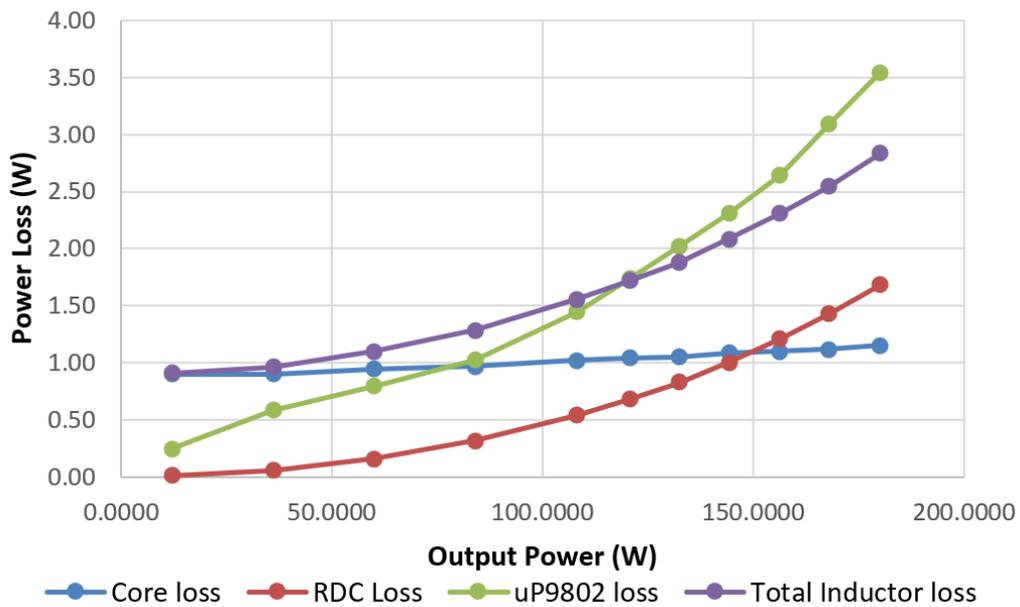
Fig. 14. Comparing the contributions of inductor and power stage losses.
