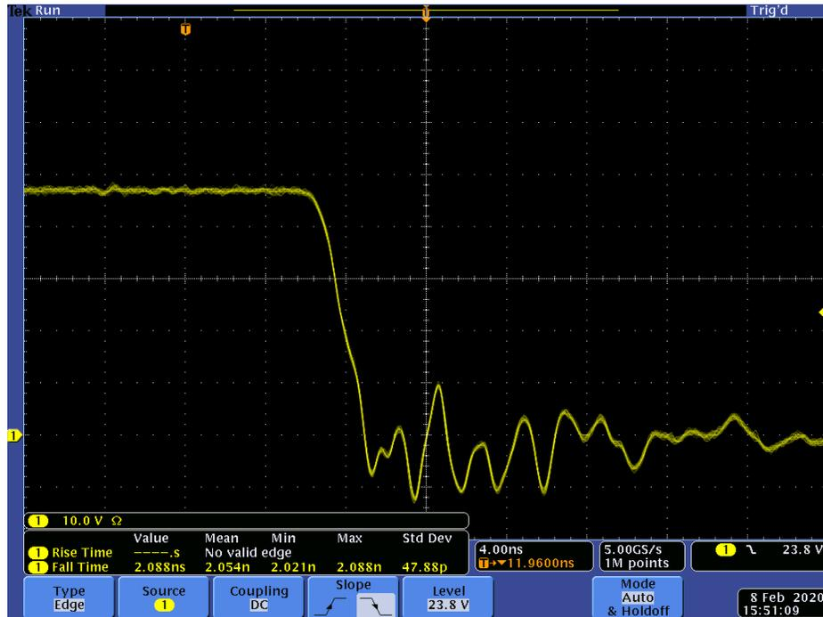
Fig. 13. Fall time measured for the uP9802Q on the test board.
