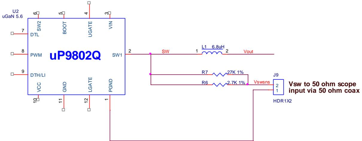
Fig. 11. 50-Ω measurement technique.
