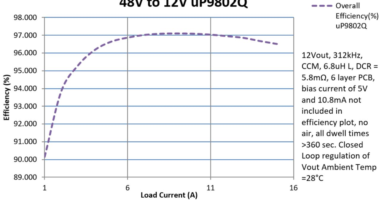
Fig. 8. Expanded efficiency plot.
