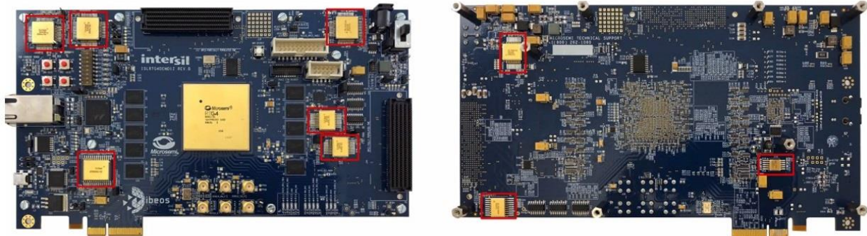
Fig. 6. With permission from Microchip Technology and in collaboration with Ibeos, Renesas modified Microchip's RTG4 development board schematic and layout, replacing its power solution with a fully QML-V qualified power solution. The Renesas regulator ICs used to generate the rails required by the RTG4 FPGA are shown in the diagram (a) and the chart (b) with photos of the development board below them (c).
