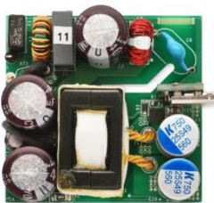
Fig. 2. Power Integrations offers two reference designs that demonstrate the highly integrated USB PD 3.0 + PPS adapter solutions enabled by the InnoSwitch3-PD ICs.
