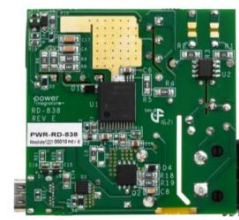
Fig. 2. Power Integrations offers two reference designs that demonstrate the highly integrated USB PD 3.0 + PPS adapter solutions enabled by the InnoSwitch3-PD ICs.
