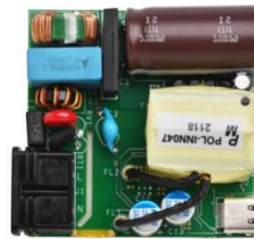
Fig. 2. Power Integrations offers two reference designs that demonstrate the highly integrated USB PD 3.0 + PPS adapter solutions enabled by the InnoSwitch3-PD ICs.
