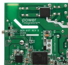
Fig. 2. Power Integrations offers two reference designs that demonstrate the highly integrated USB PD 3.0 + PPS adapter solutions enabled by the InnoSwitch3-PD ICs.
