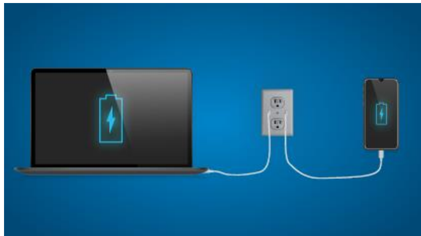
Fig. 17. Two InnoSwitch3-Pro ICs connect through a low-pin-count USB-PD controller and dynamically adjust output voltage and current. For example, when a laptop is plugged into either of the two ports, it can be charged at 65 W. When a mobile phone is then plugged into the other port, it can be charged at 20 W while the laptop is automatically adjusted to 45-W charging.
