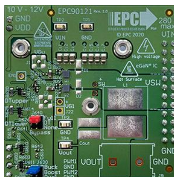
Fig. 2. Measuring 2 in. x 2 in., the EPC90121 development board contains two EPC2050 GaN FETs in a half-bridge configuration with the onsemi NCP51820 gate driver. It also contains all critical components and the layout supports optimal switching performance. Additionally, there are various probe points to facilitate simple waveform measurement and efficiency calculation.
