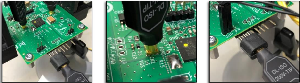
Fig. 2. The DL-ISO probe features flexible interfaces to devices under test including an MMCX connector (middle photo) for measuring gate-drive signals and a square pin header for safe high voltage (1000 V and 2500 V) measurement. Additionally high-quality coaxial leads improve EMI/RFI immunity and reduce stray noise pickup.
