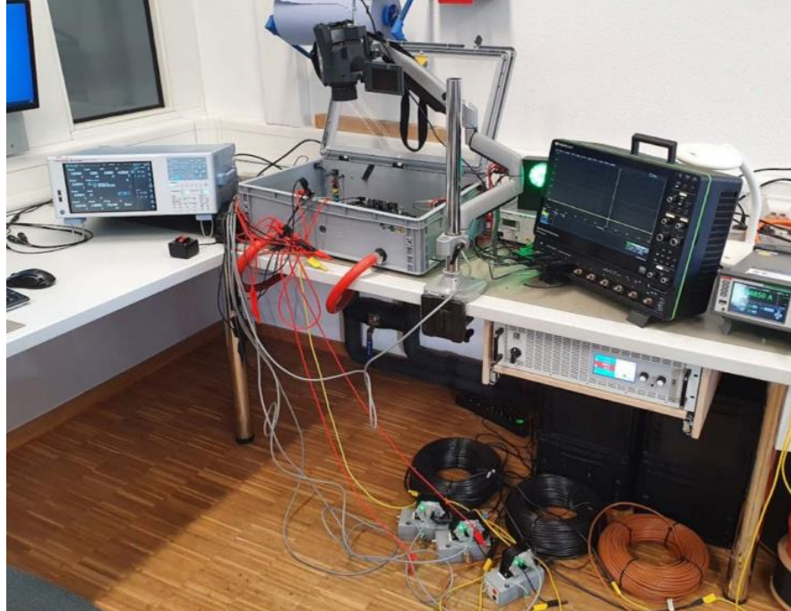
Fig. 1. The Hillcrest inverter proof-of-concept implements the company's proprietary ZVS control algorithm on a TI C2000 microcontroller and uses SCT3160KW 160-m \Omega 1200-V SiC MOSFETs from Rohm in the power stage. This inverter achieved significant reductions in losses at higher switching frequencies versus a comparable hard-switched inverter as documented in the white paper.
